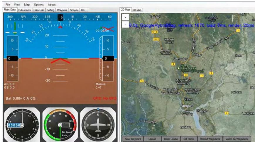
Fig.8 Ground Control System with Customized Map
